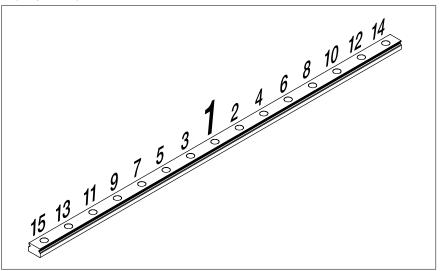
Fixing MINIRAIL guideways correctly
