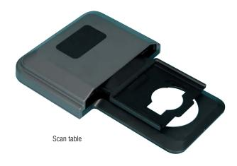
The Scan table shown is based on MINIRAIL and MINISCALE PLUS; the drive is provided by linear motors. Using these compact components reduces the weight compared with conventional constructions (ball screws and multiphase motors) by a factor of around five. The scan table is not only fast but also decidedly quiet. Precision in the smallest area - reproducible with an accuracy of several microns.
