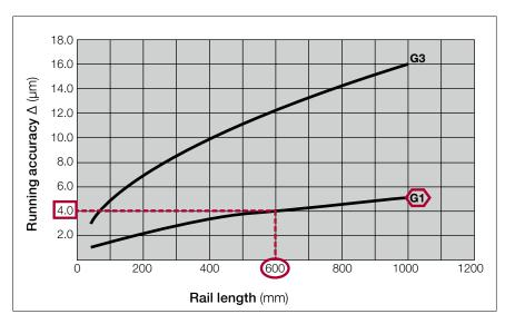
Example according to the diagram: A rail length of 600 mm and accuracy class G1 results in a maximum permissible deviation of  $4.0~\mu m$
