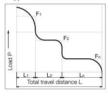
The loads (F) acting on a linear guideway system are subject to frequent fluctuations during operation. This set of circumstances should be taken into account when calculating service life. The varying load absorption of the guideway at varying operating conditions during the travel distance is described as being the dynamic equivalent load P.
