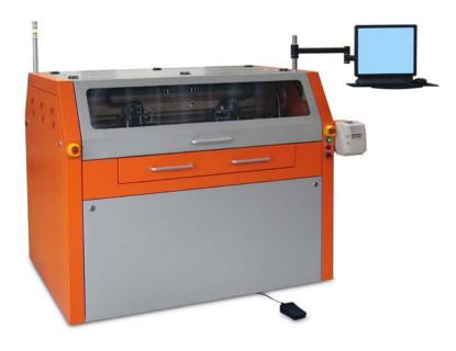
The flying probe test system
