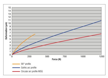
Comparison of the rigidity of structurally identical MINISLIDE size 9-80.66 with different contouring of the guideway tracks. The circular arc profile of MSQ results in the lowest deformation and therefore the highest rigidity
